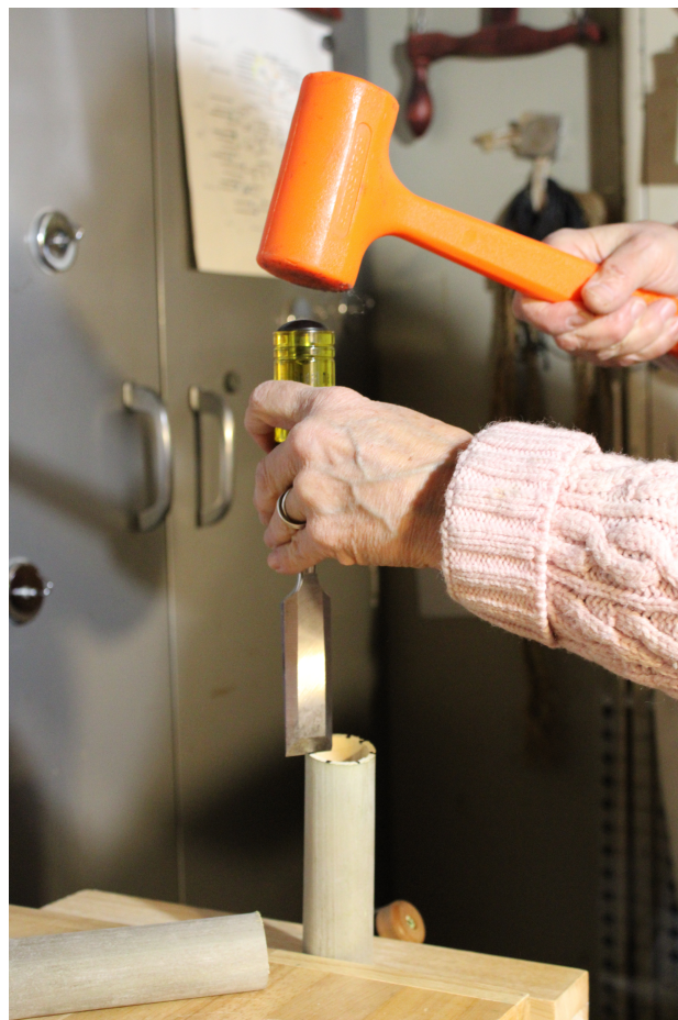
Photo above shows position of bamboo and chisel when splitting or hand sawing.
